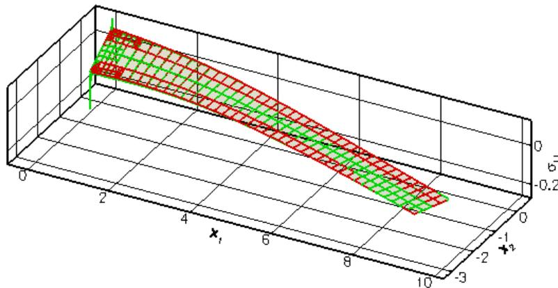
Figure 1.3: Comparison of the computed distribution of the 'horizontal' stress (in green) against the approximate analytical solution (in red).
