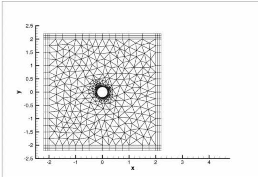
Figure 1.3: The computational domain used in the example problem.
