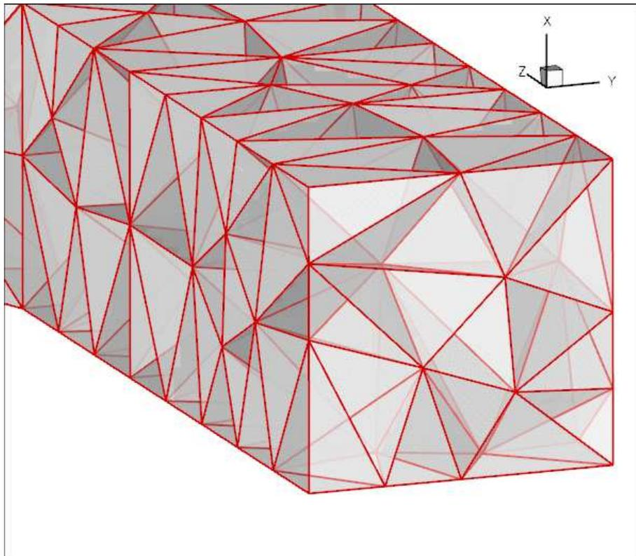
Figure 1.5: Plot of the mesh generated by tetgen.
