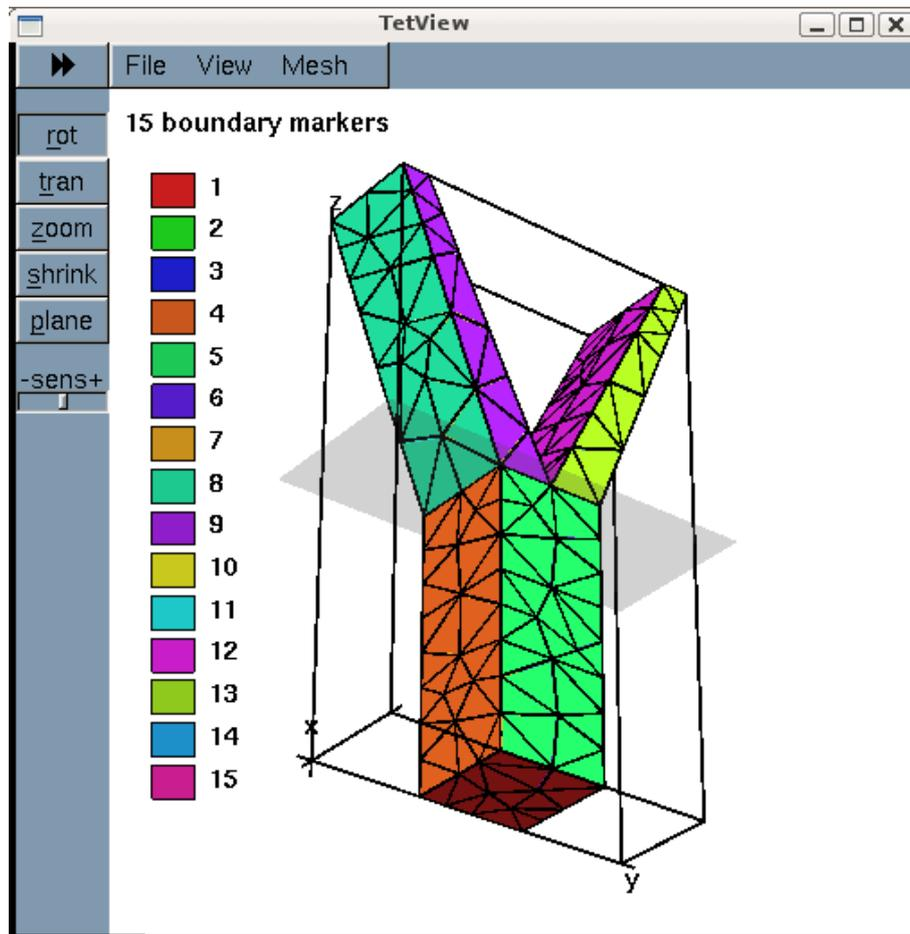
Figure 1.3: Plot of the mesh, generated by tetgen.
