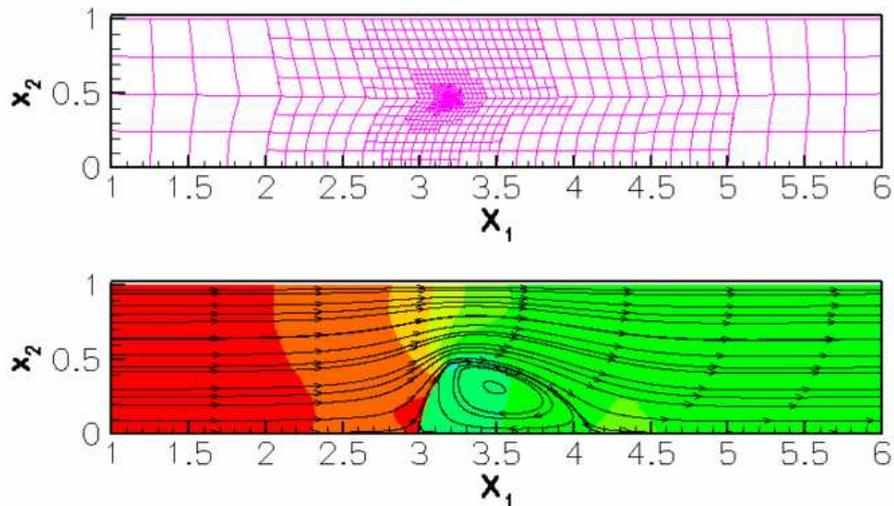
Figure 1.3: Mesh (top) and flow field (bottom).
