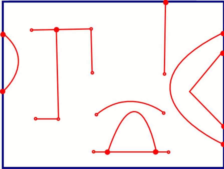
Figure 1.1: The `TriangleMeshOpenCurve` object allow us to define domains with internal boundaries. The internal boundaries are shown in red. Notice the connections of the internal boundaries with other boundaries. The connections are shown with filled small circles.
