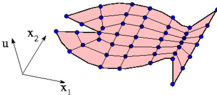
Figure 1.13: Fish-shaped domain discretised with four-node quadrilateral
