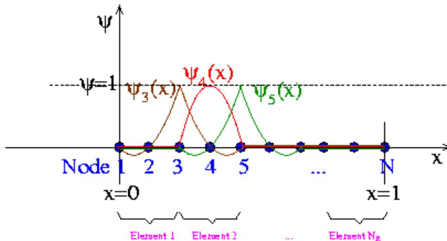
Figure 1.6: (Global) quadratic finite-element basis functions in 1D.
