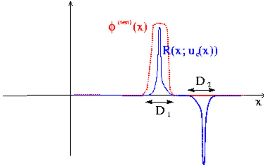
Figure 1.2: Residual (blue/solid) is nonzero only in two small sub-domains. A suitably constructed test function with finite support (red/dotted) is sufficient to show that the candidate solution is not a weak solution.
