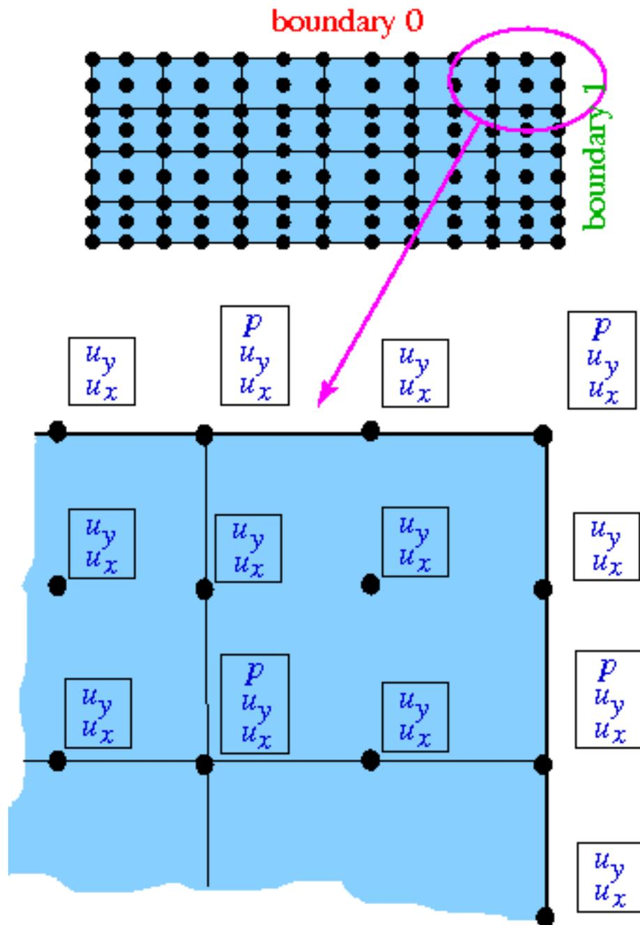
Figure 1.3: Sketch of a problem that is subject to flux-type boundary conditions along boundaries 0 and 1. The sketch illustrates the degrees of freedom at each node before any FaceElements are attached.
