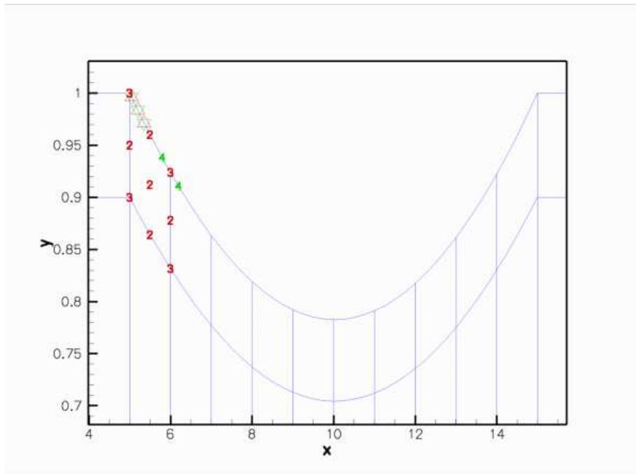
Figure 1.3: Animation of the Data values that affect the fluid traction that the adjacent fluid elements exert onto the various `FSIHermiteBeamElements` in the wall mesh. (The fluid elements are 2D Taylor-Hood elements.)
