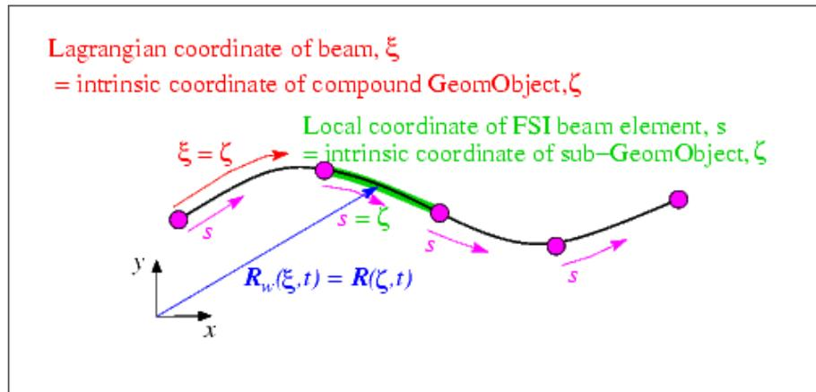
Figure 1.1: Sketch of the various coordinates and GeomObjects. The (continuous) beam is parametrised by its Lagrangian coordinate  $\xi$  which doubles as the intrinsic coordinate  $\zeta$  for its role as a GeomObject. The (discretised) beam is a compound GeomObject, parametrised by the Lagrangian coordinate  $\xi$ ; its constituent FSI beam elements are sub-GeomObjects that are parametrised by their local coordinates,  $s$ .
