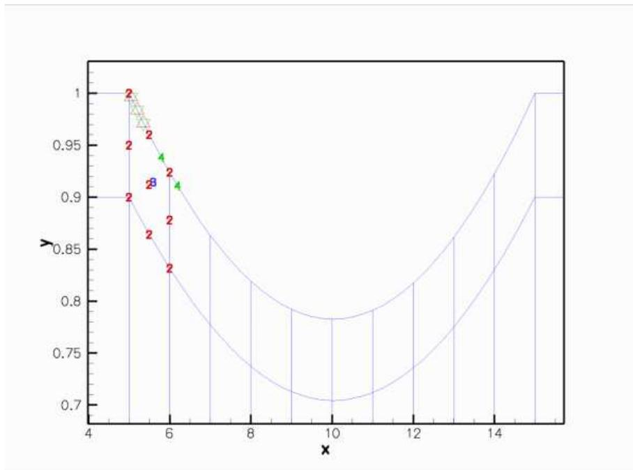
Figure 1.2: Animation of the Data values that affect the fluid traction that the adjacent fluid elements exert onto the various `FSIHermiteBeamElements` in the wall mesh. (The fluid elements are 2D Crouzeix-Raviart elements.)
